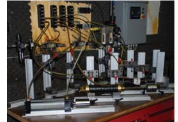
Cylinder test station
