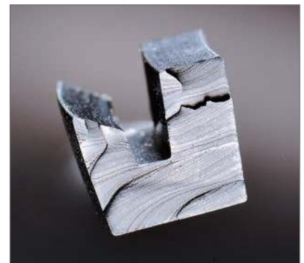
The seal after 1 million cycles shows virtually no wear.
