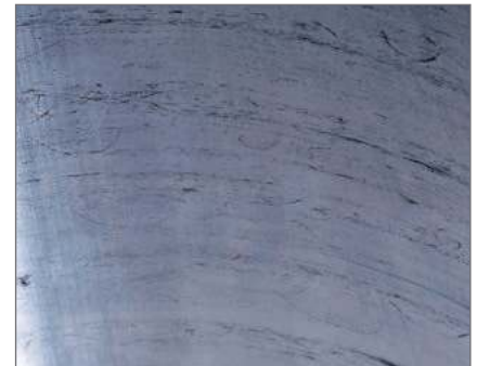
PolySlide cylinder wall surface showed minimal wear.
